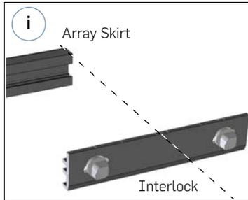
Position an Interlock with the Key side towards the Array Skirt, aligning the end of the Array Skirt with the center mark on the Interlock.
