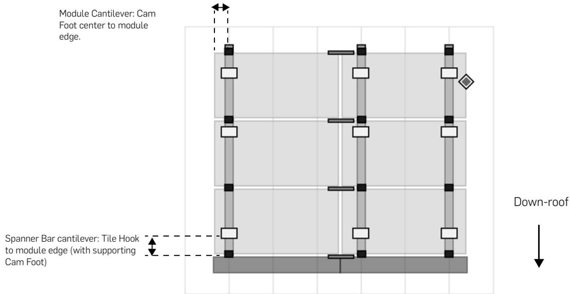
**Spans are site and project-specific.** Field installers should keep the span allowances in mind for each job, as they may need to re-configure an array due to unexpected conditions at the job site.
