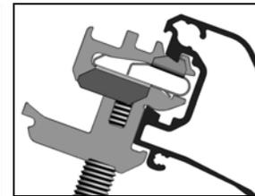
Bottom edge of Array Skirt should be flush against Cam Foot Rockit.
