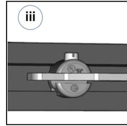
Using either the Zep Tool or the Flat Tool (shown), lock the Ground Zep into place by turning 1/4 turn clockwise. After the Ground Zep is turned 90 degrees, the set screw should be pointing straight up.
