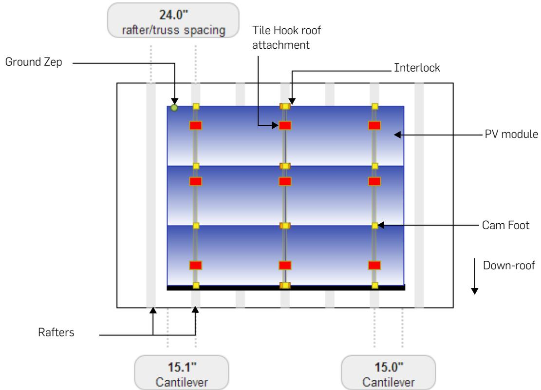
The Zepulator centers the array in the specified roof mounting area.
