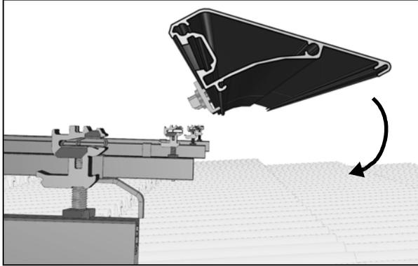
Array Skirt can be shifted to avoid conflicts between Interlocks and Cam Feet. Be sure to stay within module cantilever allowances as described in ["Spacing Rules"](#) on page 20.
