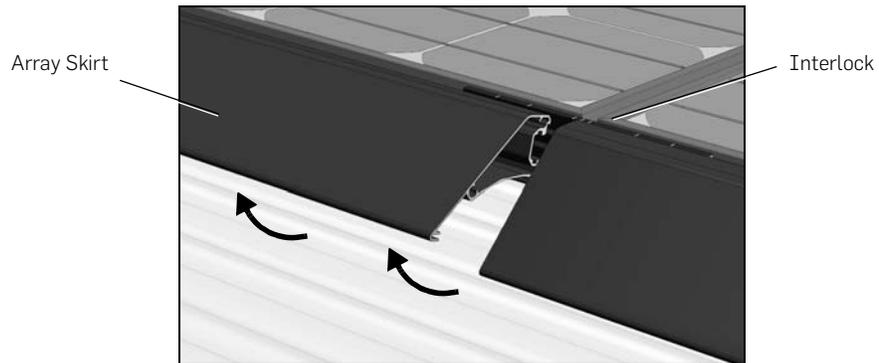
4. The Interlocks are revealed with the Key side showing.
