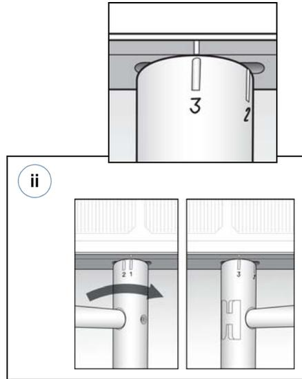
Rotate the Zep Tool from Position 1 to Position 3. **Do not over-turn.** Over-turning may prevent next row of modules from seating properly.
