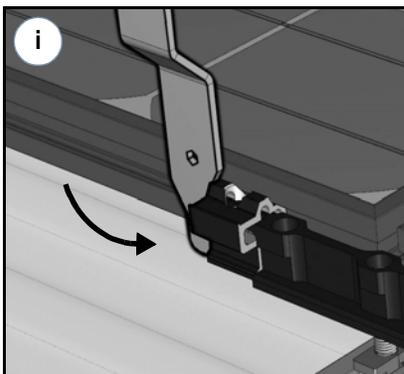
Using the Zep Tool or Flat Tool to provide leverage as needed, attach the Hybrid Interlock to the PV module frame or Array Skirt.
