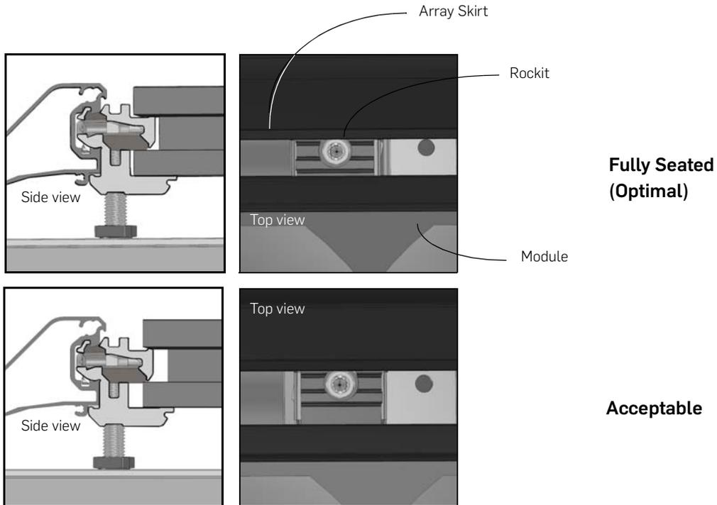
Visually check that first module is aligned and straight. Ideally, Rockit block of Cam Foot should be flush with module edge. Remove module and re-seat if needed.
