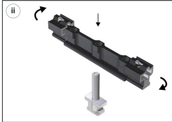
Insert the Cam Foot stud into one of the holes on the Hybrid Interlock, and spin the Hybrid Interlock to attach it.
