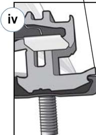
The Grip fits underneath the Array Skirt. Press upwards and pull towards you **(i)** to engage the Grip with the Array Skirt **(ii)**. Slide the Grip snugly around the right side\* of the threaded stud **(iii)**. Make sure the Grip notch also fits into the corresponding notch in the Rockit **(iv)**.
