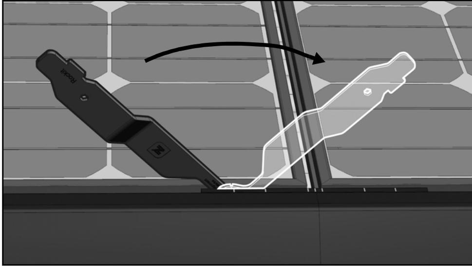
3. Remove Array Skirt sections by rotating them up and off the first-column Cam Feet.
