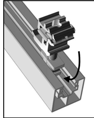
Attach first row of Cam Feet 1.25 inches from Spanner Bar ends, measuring to the center of the Cam Foot threaded stud. (Minimum distance is 1/2")
