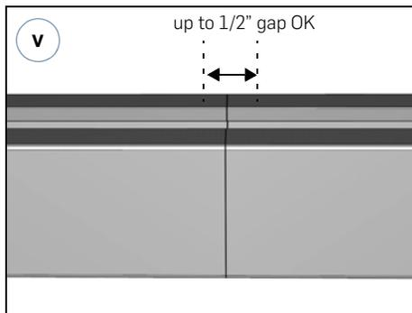
Spanner Bars should be flush when fully spliced, tolerance of +/- 1/4".
