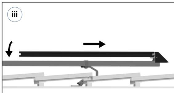
Rotate module downward almost flat, while pushing module onto tongues of Cam Feet and Interlocks. Frame engages at 15 degrees.
