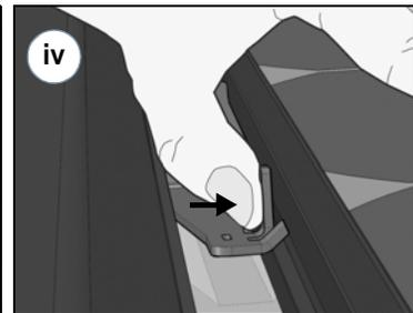
Press down (iii) and then inwards (iv) on the tail of the T-Lock to fully secure the Array Skirt.
