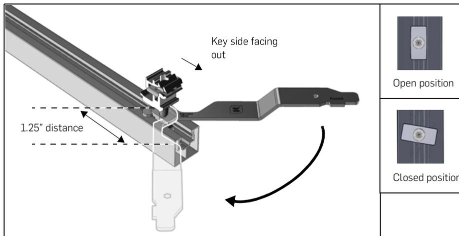
Tighten Cam Foot base 100 degrees, using Flat Tool.
