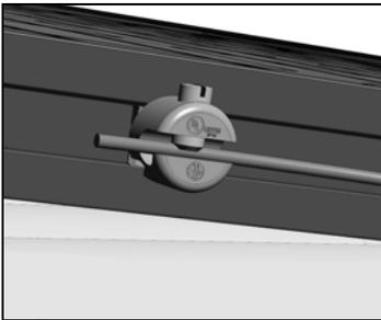
Insert solid copper ground wire into the ground wire retention slot and turn the set screw with a flat-bladed screwdriver until the ground wire is captured by the set screw. Torque the set screw as follows:
