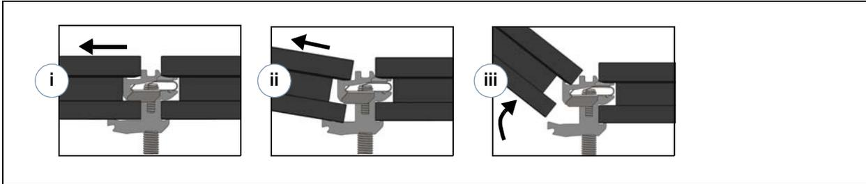
**6. Remove mid-array Interlocks from next row of modules, using Flat Tool.**
