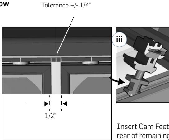
Align module with Interlock timing marks. Allow 1/2" gap between modules.
