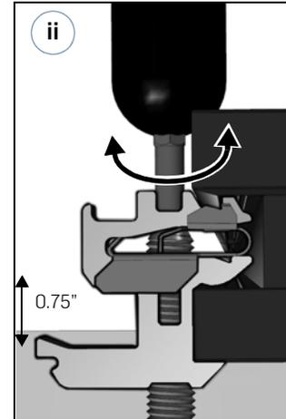
**Ensure that all modules in first column are level.** This will aid in keeping the rest of the array true.
