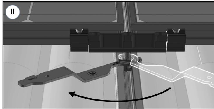
Secure Cam Foot base to Big Foot using Flat Tool, turning 100 degrees. Keep the center of each Rockit minimum 2 inches from module corner.
