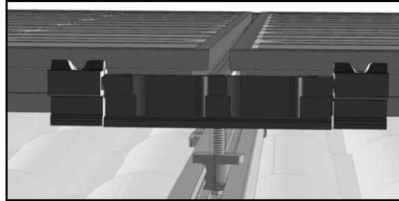
The Hybrid Interlock has a dual function: attachment to the Comp Mount and structural connection between modules.
