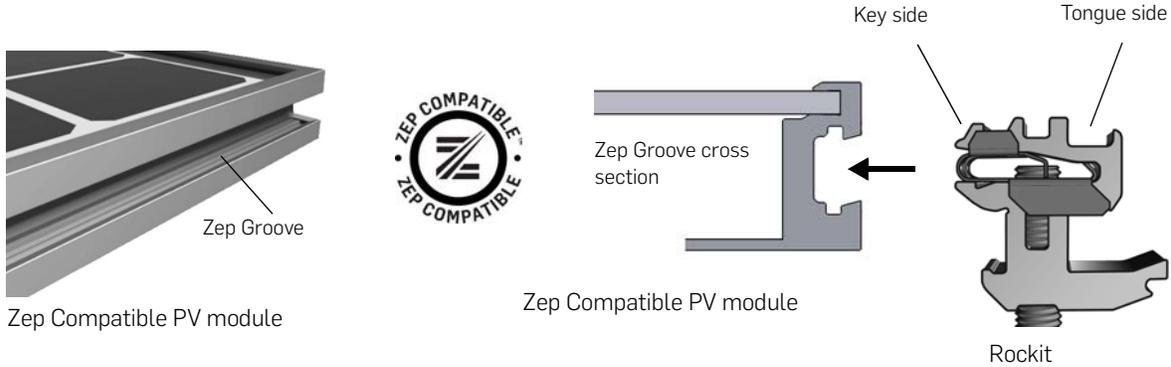
For example, the "Rockit" is a hardware feature used to secure PV modules to the roof attachments. The Rockit fits into the Zep Groove on both sides: The Key side inserts, while the Tongue side receives.
