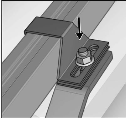
Torque the carriage bolt on Spanner Clamps going up the column.
