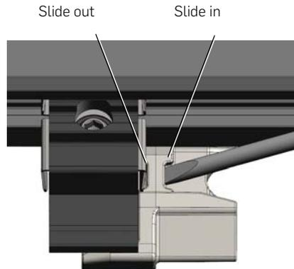
Apply screwdriver to one side of position notch for leverage.
