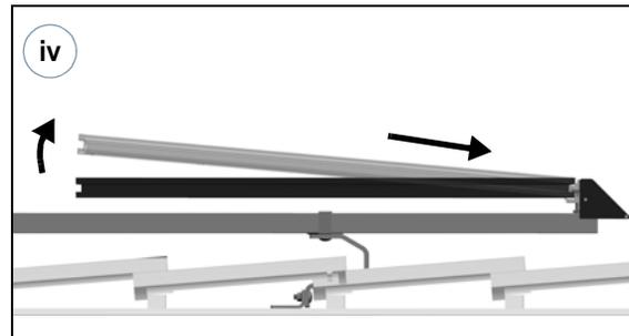
If needed, lift module up slightly, and apply force towards Cam Feet to seat the module completely.
