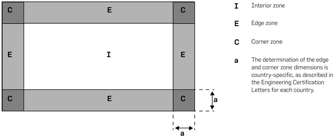
When generating array layouts, the Zepulator assumes that the entire mounting area is within an Interior roof zone. For detailed examples showing applications of array layouts within edge and corner roof zones, and how to determine the dimensions of these zones, please refer to the Engineering Certification Letter and Span Tables document that is appropriate for the project location. This document is available on the Zep Solar web site.
