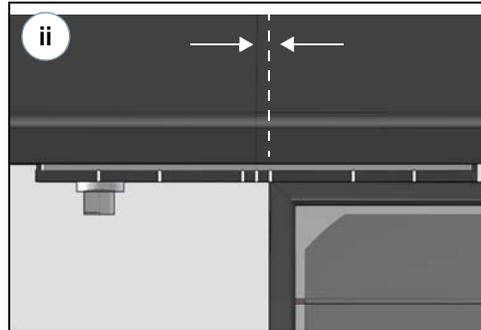
Adjust module edge alignment using Interlock timing marks. (If Interlock is offset to avoid Cam Foot conflict, align module using Array Skirt.)
