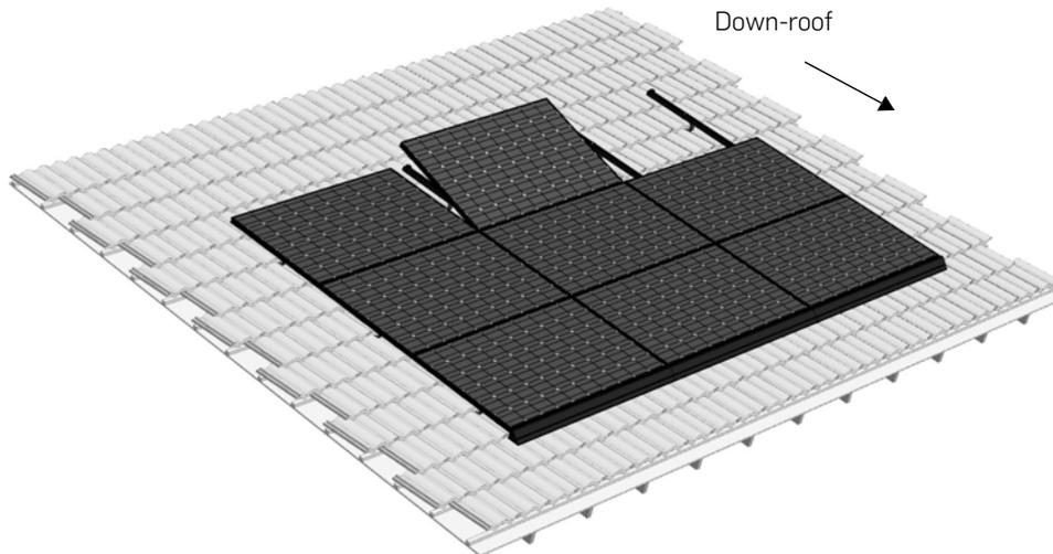
Install remaining modules, row by row. True and level the array as you go. Attach Interlocks and Cam Feet as before. Clip and secure wires for each row before moving on to the next row.
