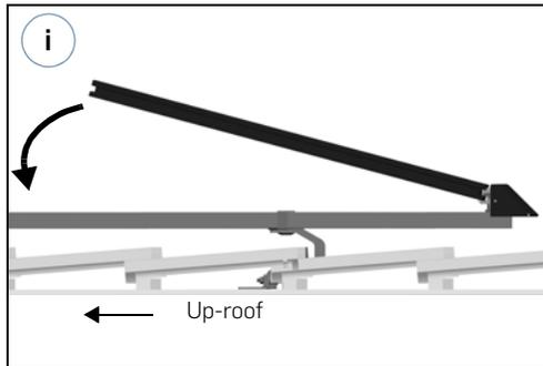
Place first module on Tongue side of Cam Feet and Interlocks at a steep angle.
