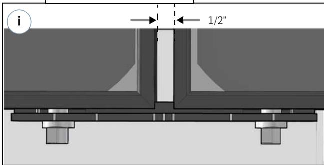
Align Interlocks with module corners using timing marks.
