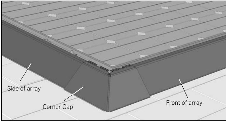
Installers have the option of attaching the Array Skirt and Corner Caps to the sides of a completed array for an enhanced visual appearance.
