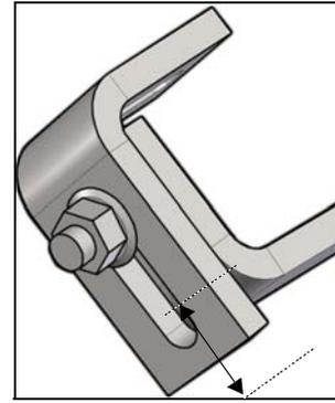
Some Tile Hooks allow adjustment of the hook depth.
