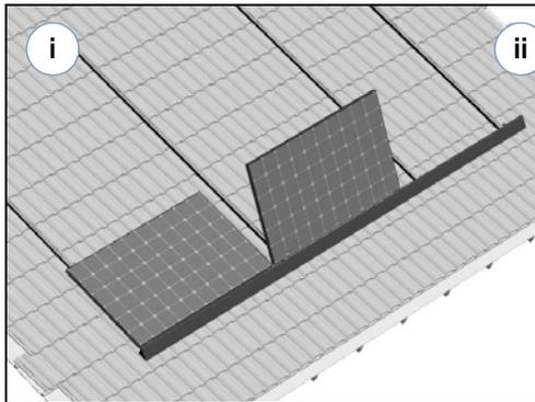
Place the second module on Tongue side of first-column Cam Feet and Interlocks.
