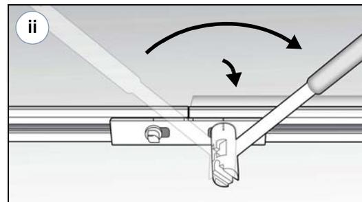
Simultaneously tighten Interlock to Position 3 (closed) while rotating next section of Array Skirt into place on the first-column Cam Feet.
