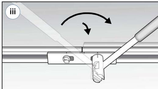
Attach the second Array Skirt section, and tighten the Interlock on the second side. **Skirt will not be flush at the bottom until Zep Tool is fully turned to Position 3.**
