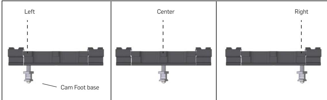
When threading the Cam Foot base for a Hybrid Interlock, choose the hole that best centers the Hybrid Interlock between Array Skirt sections or modules. For Interlocks connect PV modules within the field of the array, only the center hole may be used.
