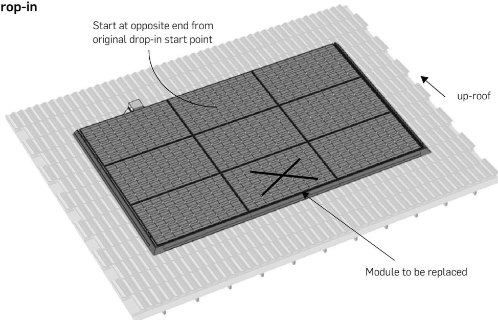
2. **Disconnect wires from first module to be removed.**
