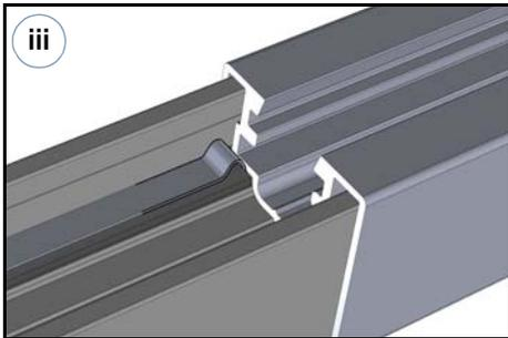
Slide the Splice Kit into the first Spanner Bar until the ridge in the Splice Kit meets the Spanner Bar edge as shown.
