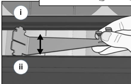
Engage one side of the T-Lock head with the Zep Groove (i). Then snap the Array Skirt onto the T-Lock from the other side (ii).
