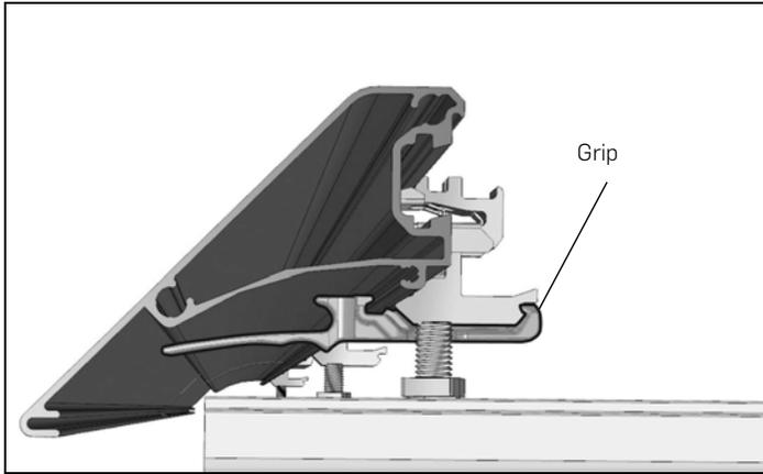
To fully secure the Array Skirt, a Grip is fitted around the Rockit of **every** first-row Cam Foot.
