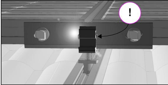
A Cam Foot-Interlock conflict occurs when the location of a Cam Foot coincides with the location of an Interlock.
