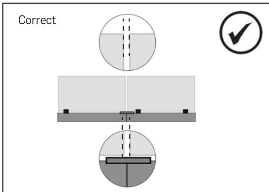
Gap between modules should be consistent at the upper and lower edge of each module.
