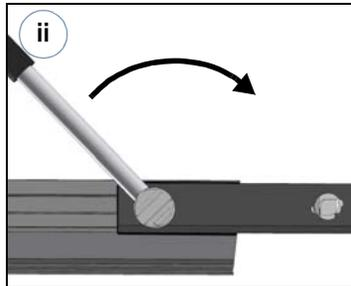
Use the Zep Tool to secure the Interlock on one side.
