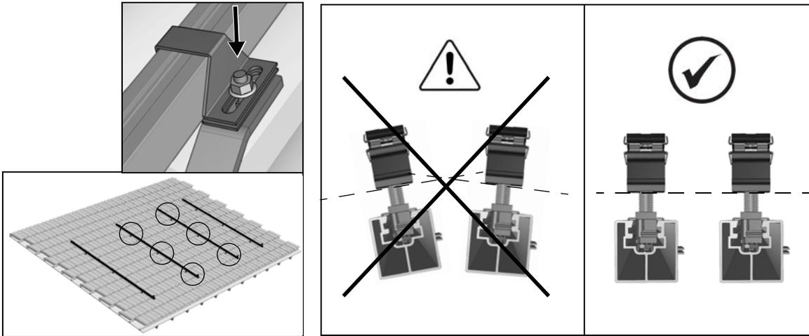
Secure Spanner Clamps going up each middle Spanner Bar.
