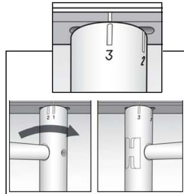
Rotate the Zep Tool from Position 1 to Position 3.
