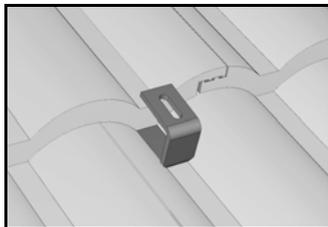
Tiles may require grinding in order to fit flush.
