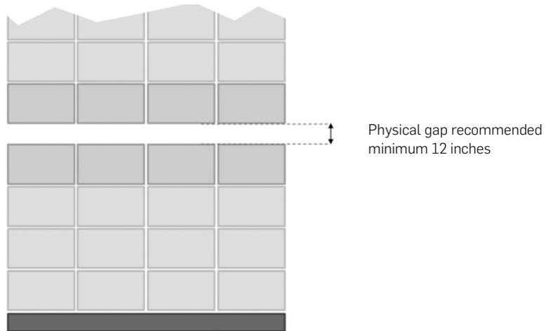
**Figure 4.13 East-West Drop-In, Thermal Expansion Gap**
