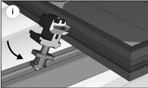
Manually insert the Key side of the Cam Foot into Zep Groove while aligning Cam Foot base with Spanner Bar channel.
