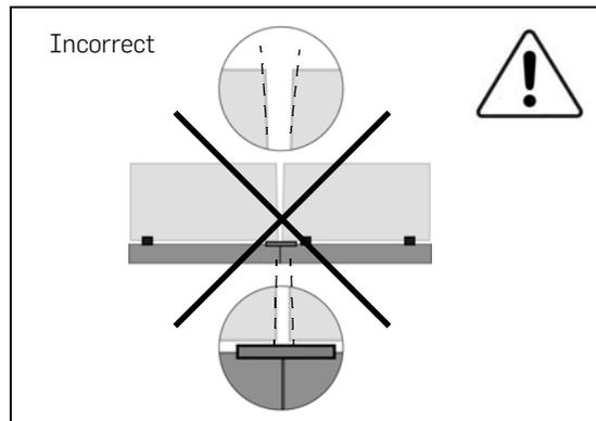
If module gap is not even, detach Cam Foot base and re-seat modules until row is straight.
