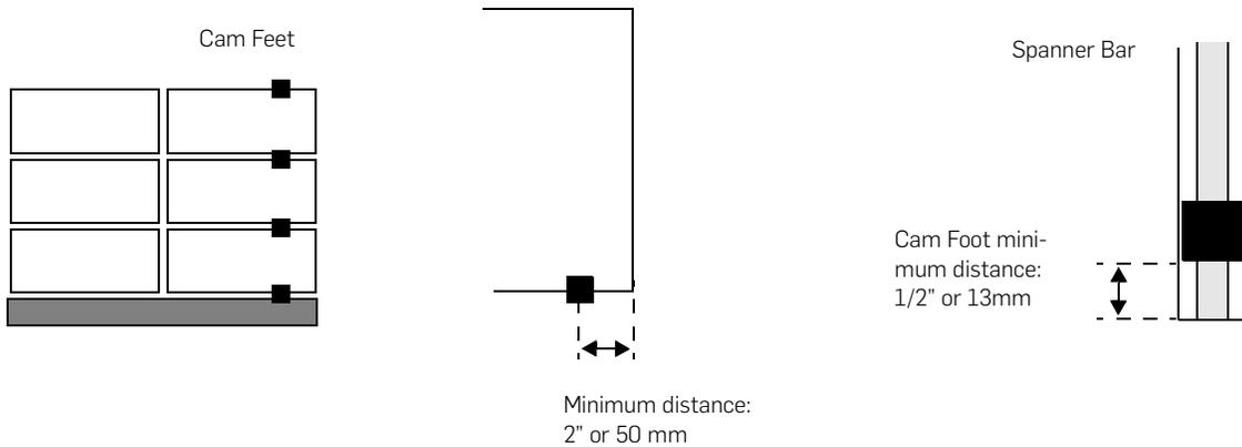
**Spacing Between Modules.** Any two modules bonded by the same Interlock should always be spaced 1/2 inch apart, with a tolerance of +/- 1/4 inch.
