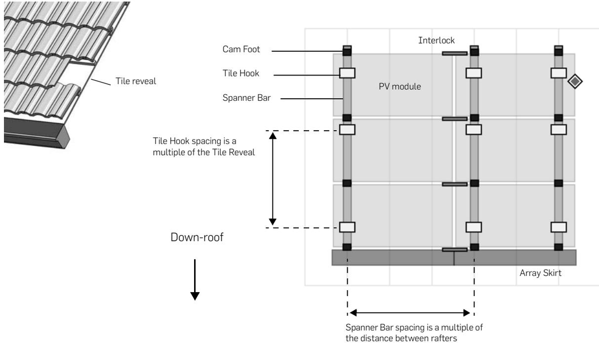
**Spacing terminology is dependent on Spanner Bar direction.** Most of the examples in this manual show Spanner Bars running North-South. However, if the Spanner Bars run East-West, then the Tile Hook spacing will refer to the the dimension that is a multiple of the spacing between rafters, and the Spanner Bar spacing will be a multiple of the Tile Reveal. See [“Engineering Rules”](#) on page 20 for more details.
