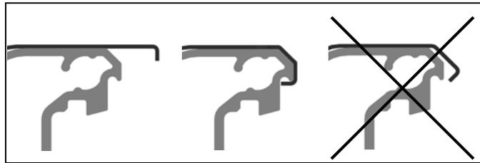
Tabs should bend tightly around the top of the Array Skirt. Use the Flat Tool to bend the tabs if needed.
