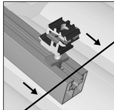
Slide middle Spanner Bars into position until Cam Feet threaded studs meet string line.
