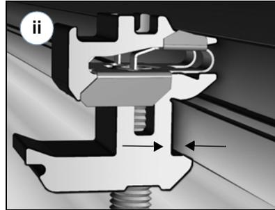
Flat face of Rockit should be flush with module frame.
