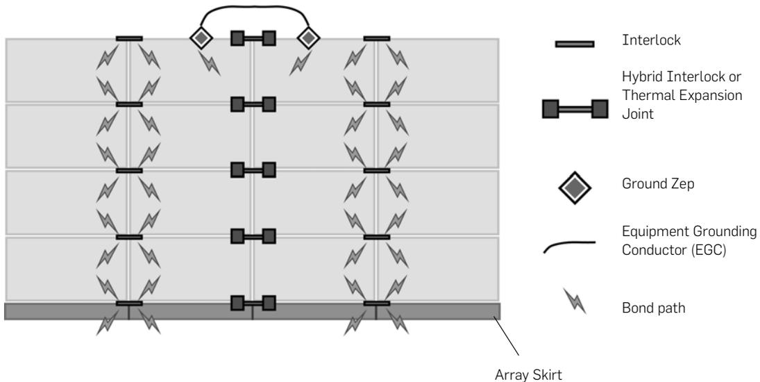
An array with a continuous column of Hybrid Interlocks (or a Thermal Expansion Joint) must be installed with a Ground Zep on either side of the column and a copper conductor wire between the two, in order to bond the two electrically isolated sub-arrays.
